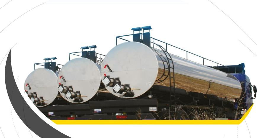
Bitumen Relay Tanker is the most versatile and functional solution with its various capacities according to your requirements and optional heating and pumping systems, for hauling bitumen, PMB, emulsion and other similar materials.
